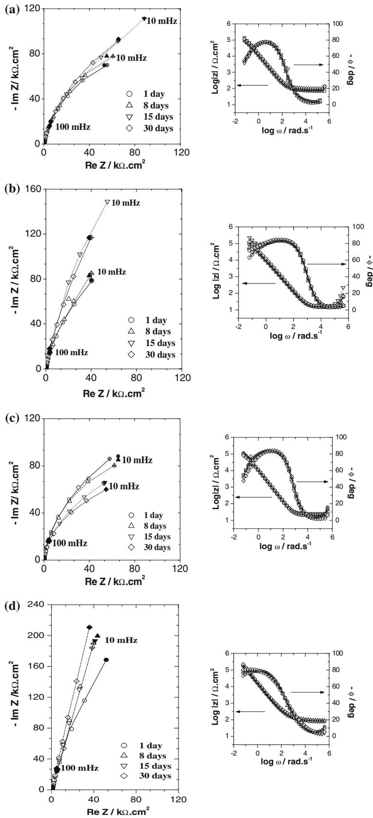
**Fig. 3** EIS diagrams of the steel bars immersed in various media: (a):  $S_1$ , (b):  $S_1 + SP$ , (c):  $S_1 + TSPP$ , (d):  $S_1 + HEDP$ . Lines represent adjustment of the experimental data
