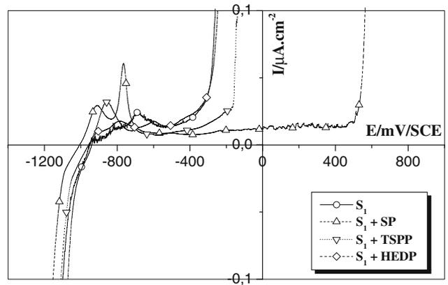
**Fig. 7** Polarization curves of steel bars immersed in  $S_2$  solution with and without inhibitors
