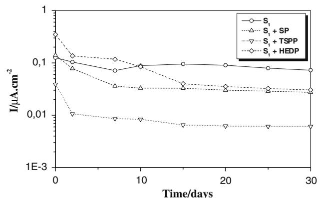
**Fig. 2** Corrosion current density versus time for bars in S<sub>1</sub> solution with and without inhibitors
