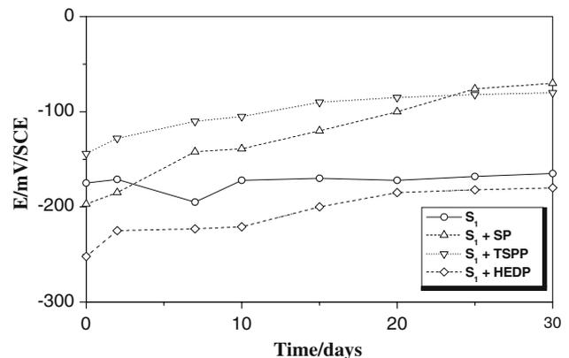
**Fig. 1** Open-circuit potential evolution for the steel bars immersed in S<sub>1</sub> solution with and without inhibitors
