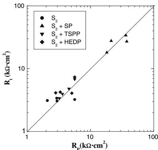
**Fig. 12** Comparison  $R_p$ – $R_t$  for steel bars immersed in Ca(OH)<sub>2</sub> sat + NaCl 0.5 M solution (S<sub>2</sub>) with and without inhibitors
