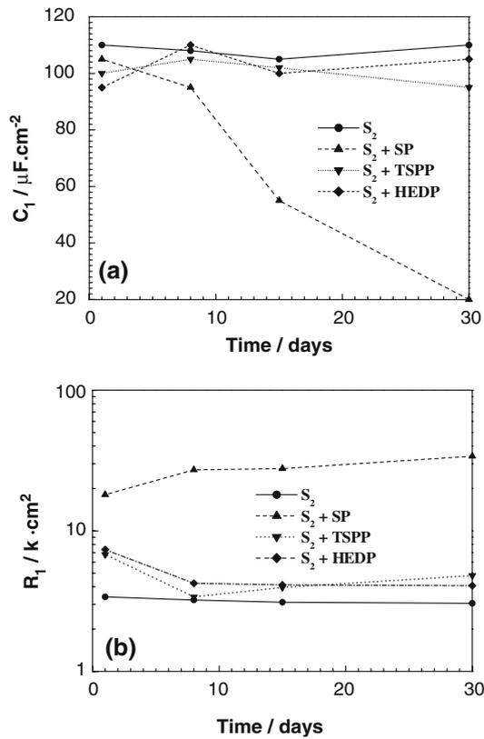
**Fig. 9** Evolution of  $C_1$  and  $R_1$  versus time of steel bars immersed in  $S_2$  solution with and without inhibitors
