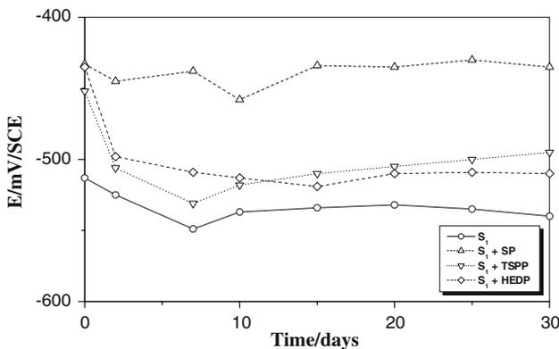
**Fig. 5** Open-circuit potential evolution for the steel bars immersed in  $S_2$  solution with and without inhibitors
