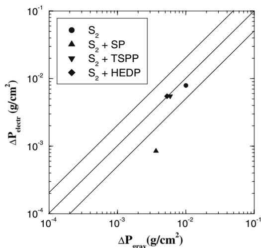
**Fig. 11** Relation between gravimetric and electrochemical weight loss of the steel bars immersed in Ca(OH)<sub>2</sub> sat + NaCl 0.5 M solution (S<sub>2</sub>) with and without inhibitors
