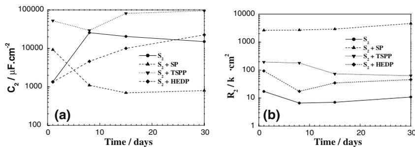
**Fig. 10** Evolution of  $C_2$  and  $R_2$  versus time of steel bars immersed in  $S_2$  solution with and without inhibitors
