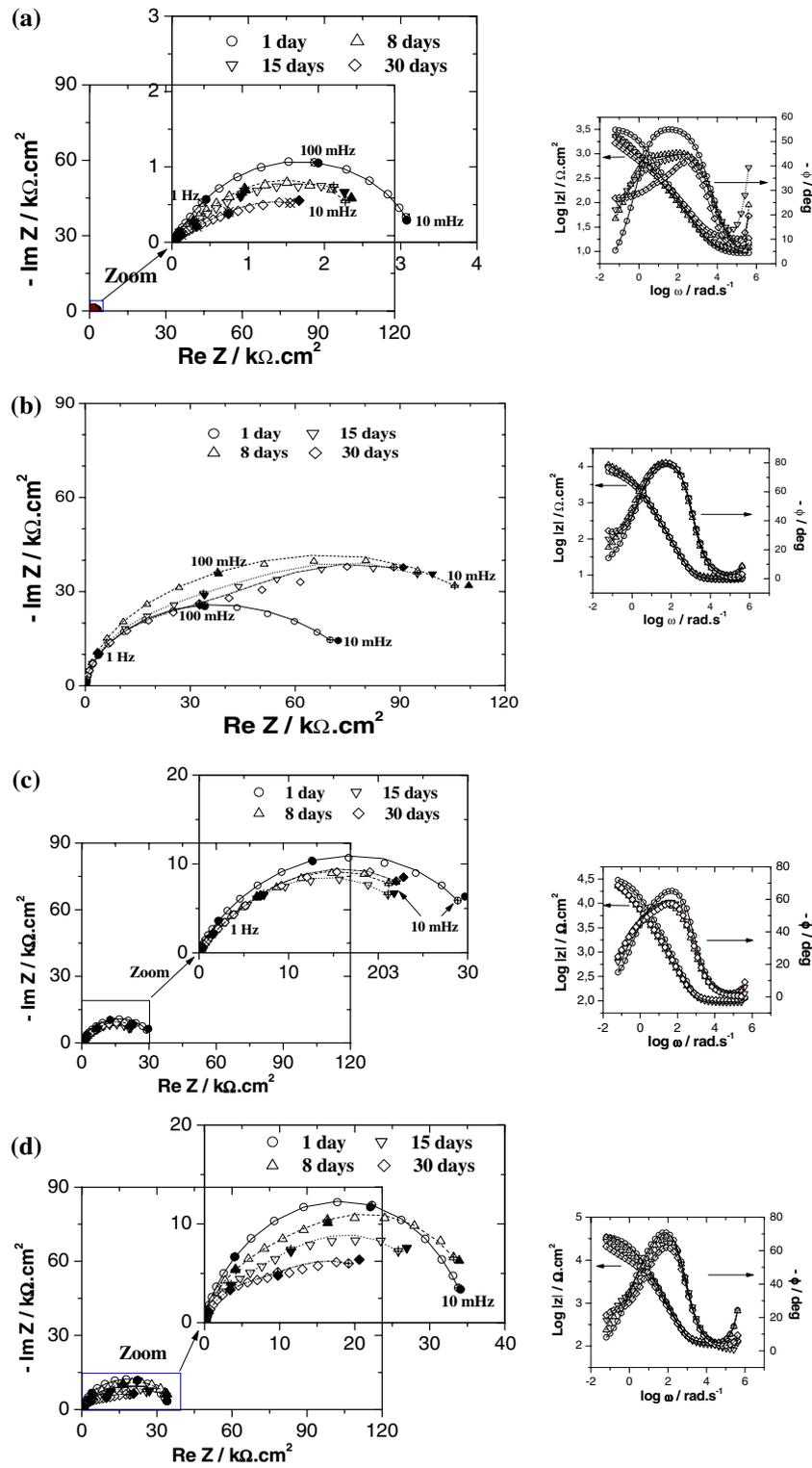
**Fig. 8** EIS diagrams of the steel bars immersed in various media: (a):  $S_2$ , (b):  $S_2 + SP$ , (c):  $S_2 + TSPP$ , (d):  $S_2 + HEDP$ . Lines represent adjustment of the experimental data
