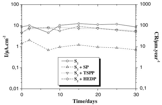
**Fig. 6** Corrosion current density ( $i_{corr}$ ) and corrosion rate ( $CR$ ) versus time for steel bars in  $S_2$  solution with and without inhibitors
