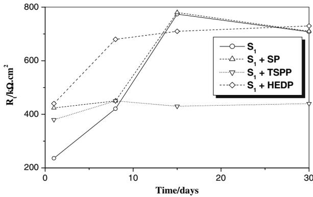
**Fig. 4** Evolution of  $R_t$  versus time of the steel bars immersed in  $S_1$  solution with and without inhibitors
